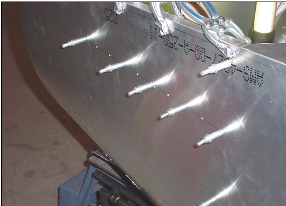
Lay out the rivet across end holes. Layout the rivet pitch. Drill an end hole in L angle, cleco in place and back drill end hole through firewall flange.
