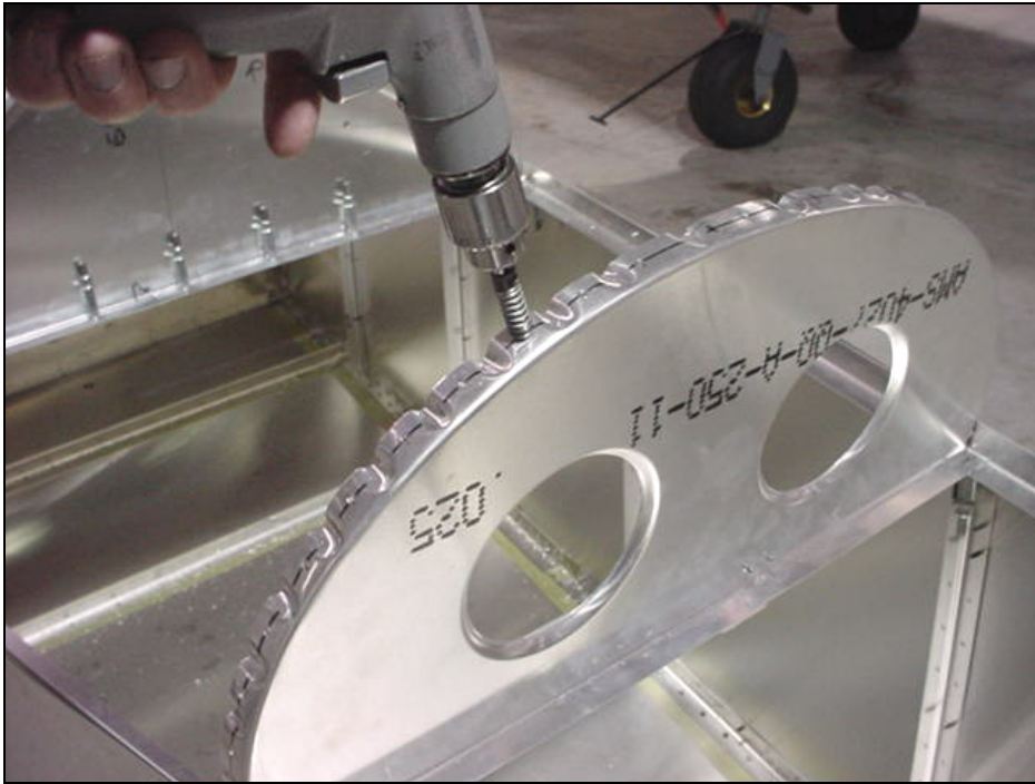
25 PILOT HOLES IN 6B12-1
