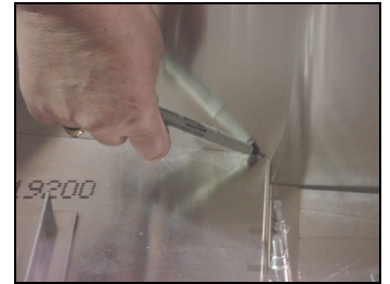
Trace around the gear channel.
