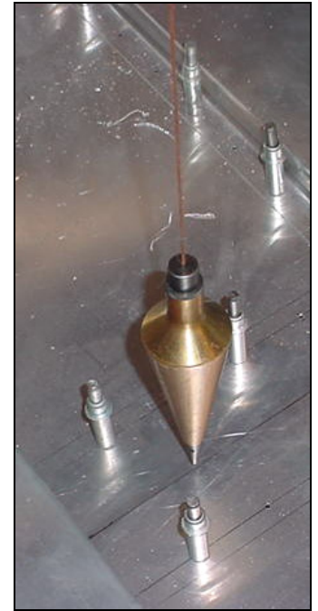
Aircraft center line on cabin floor.
