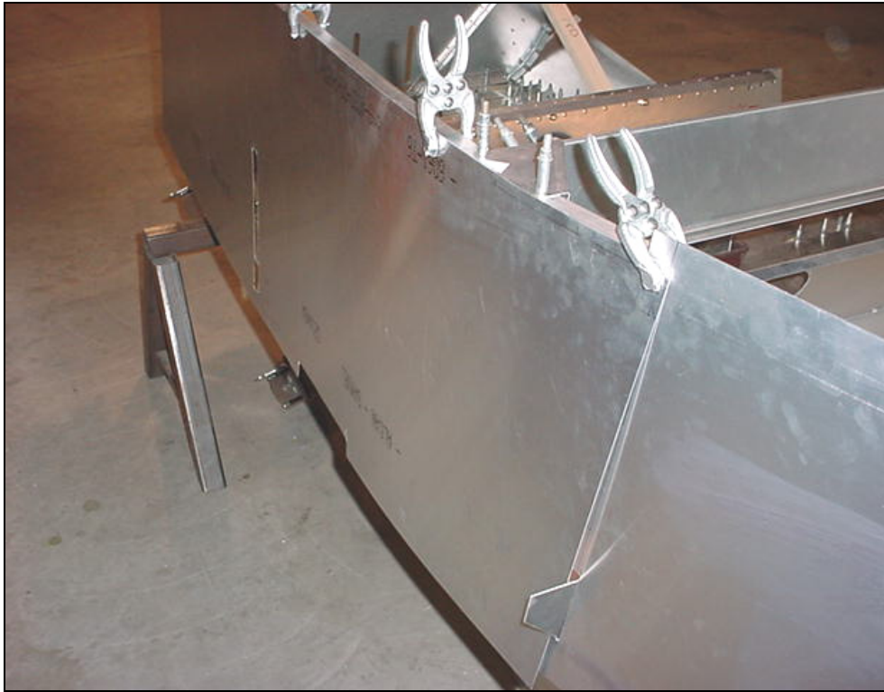
Detail of left overlap. Skins overlapped approximately 24mm
