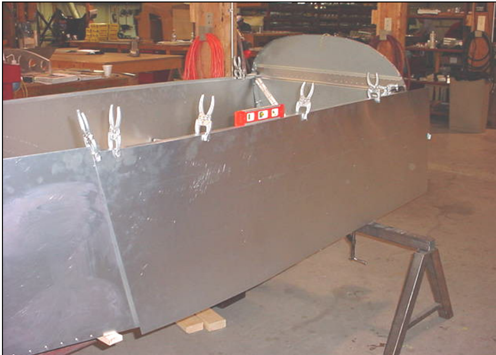
Detail of right side. Overlap is the same along the length of the overlap.
