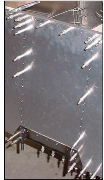
Rivet lines on outboard side of skin.
