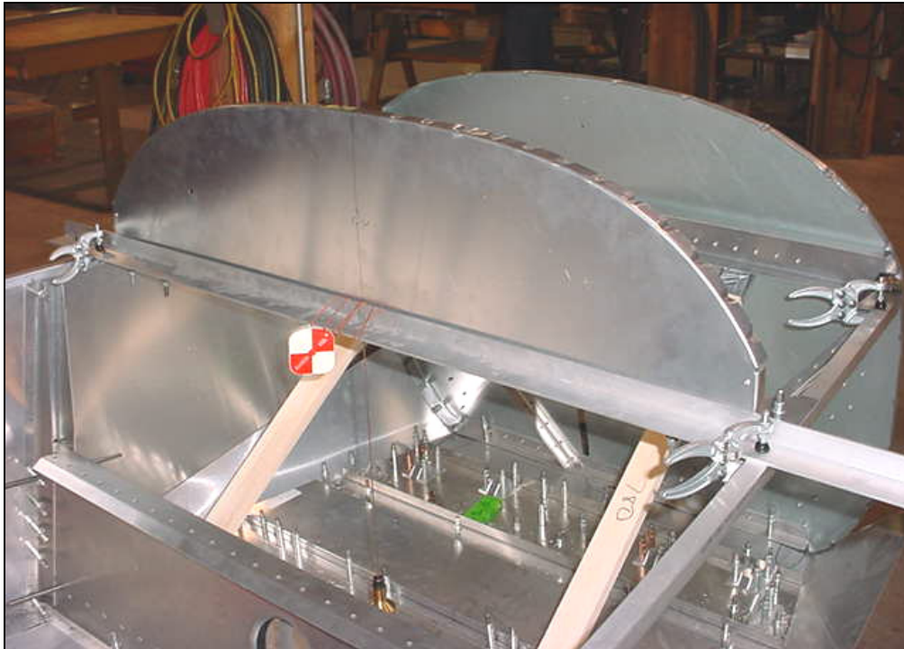
Plumb center lines.
