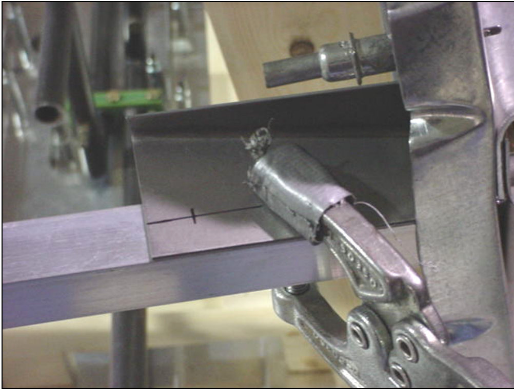
Detail of right side: Longeron clamped underneath the Upper Engine Mount Fitting 6B6-4.
