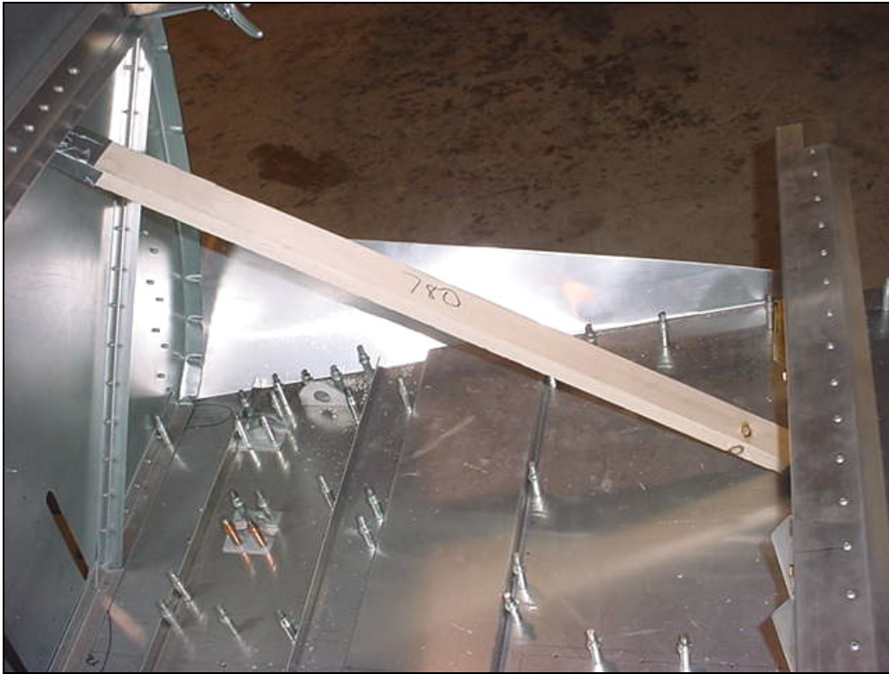
Firewall support. Furring strip (1x2 board) approximately 780 mm long, 2 required.
