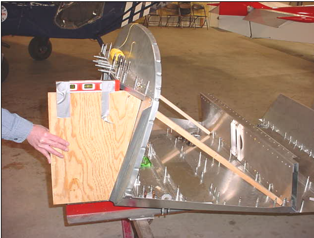
Re-check the angle of the firewall, and plumb line.
