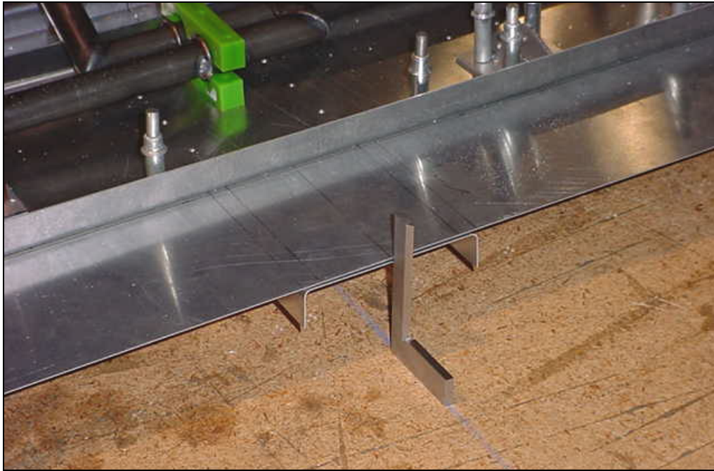
Detail of chalk line and aircraft center along front edge of cabin floor.
