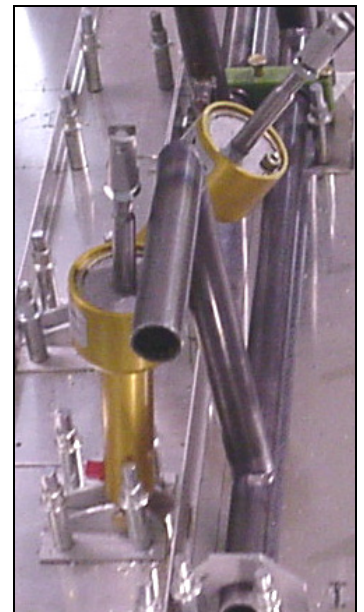
Check that the base of the master cylinder fits between the supports.
