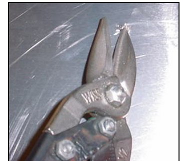
Cut out the opening.
