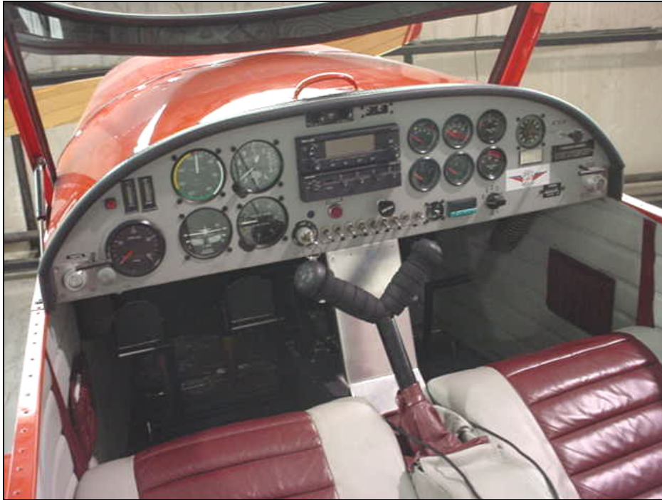
Center Console for mounting a 3-way fuel selector.
