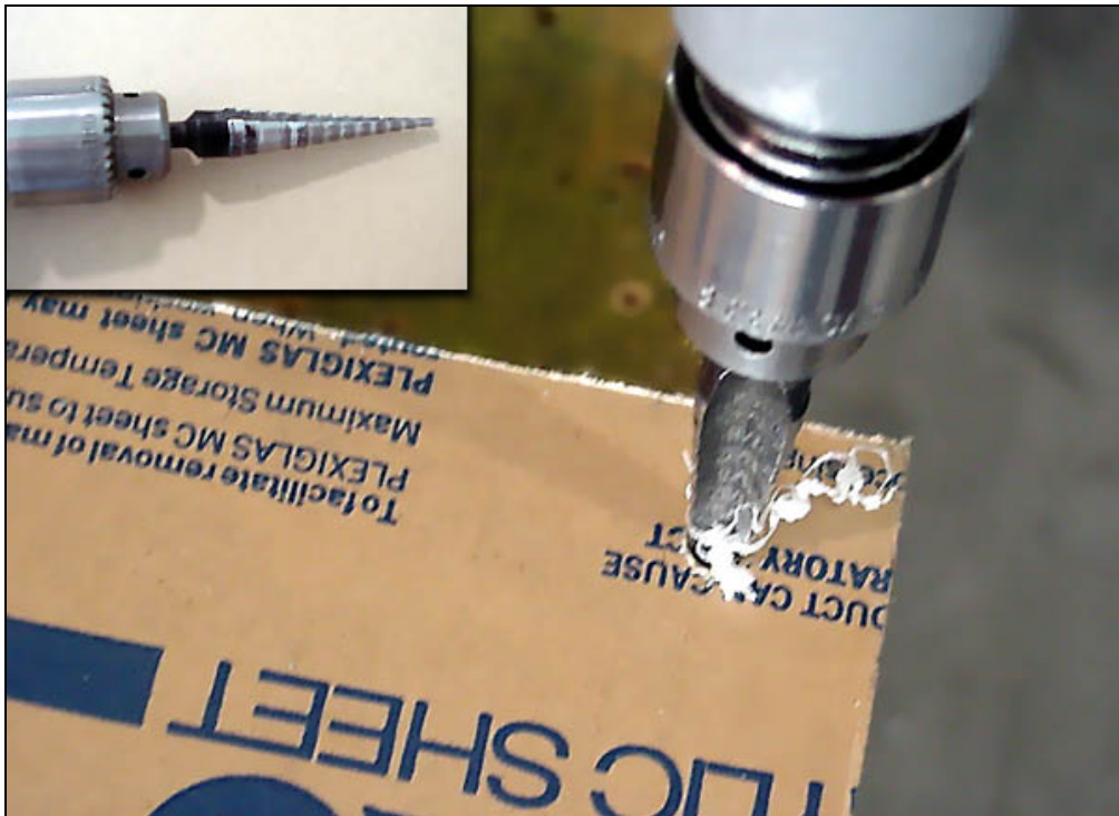
Uni-bit or step drill to open up the pilot holes in the bubble canopy.
