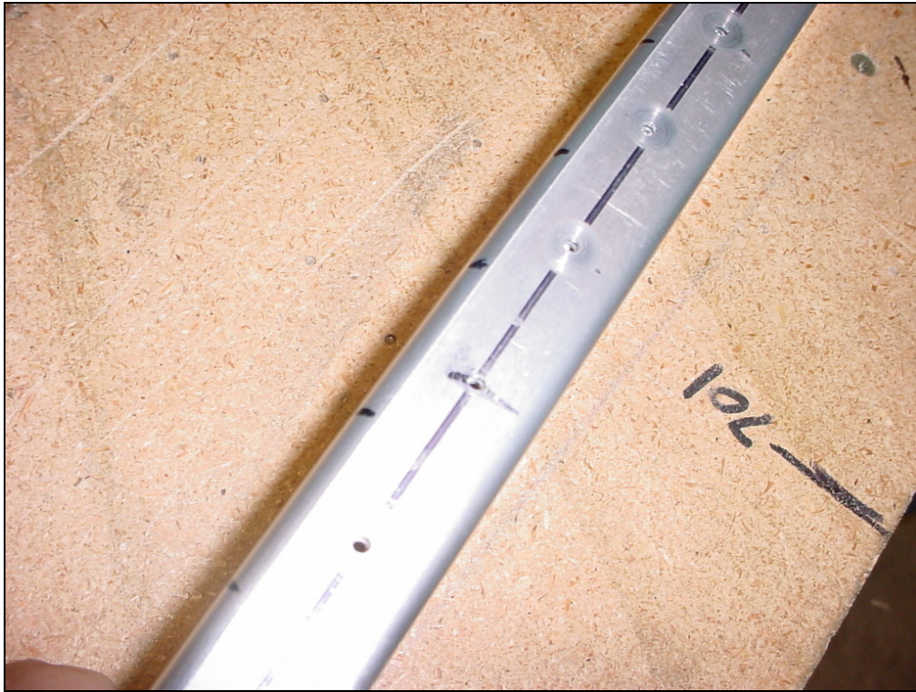
Top rivet line between the crimps.
