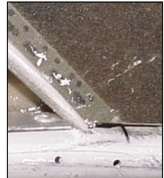
With a file open the hole along the bottom and top (elongated hole for cable housing)
