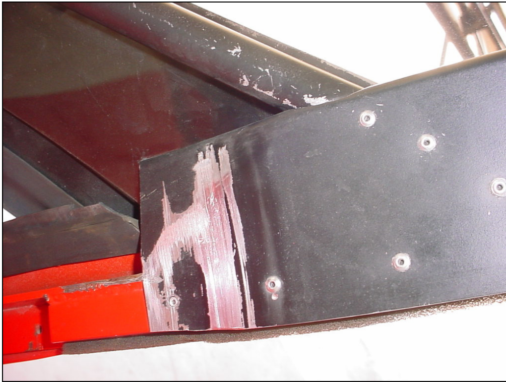
3 rivets A4 inside flashing to the front canopy tube 6C3-2
