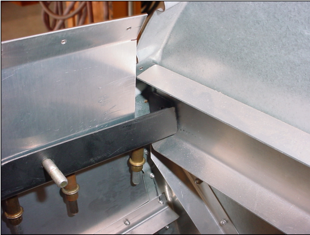
Taper the top corner of the firewall reinforcement 6B7-2
