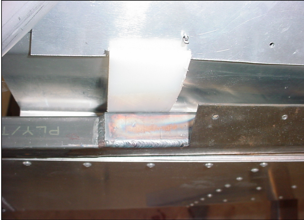
Right side. Shave down the thickness until it fit without forcing.
