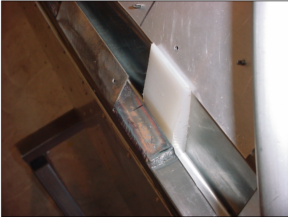
Nylon 66 material in line with the square tube of the canopy frame.
