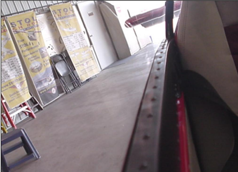
Stretch the top flange of the inside flashing to follow the curvature of the fuselage.
