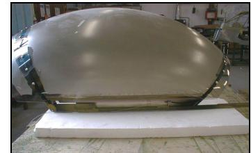
Note: Bottom edge of the canopy does not have to be parallel with the longerons.
