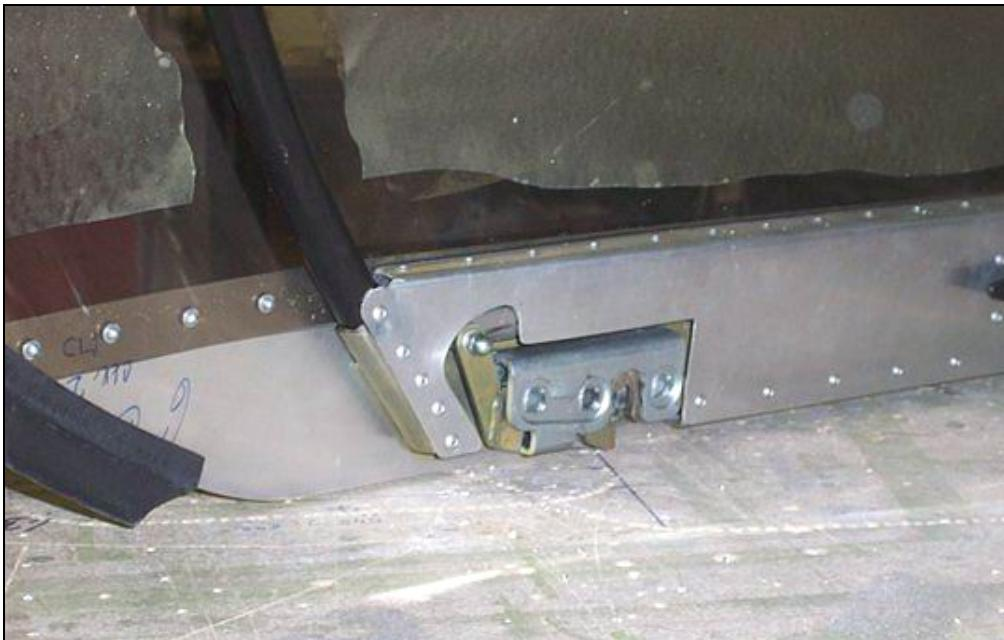
Alternative: Larger cutout on inside flashing 6C3-5 to make room for the latch
