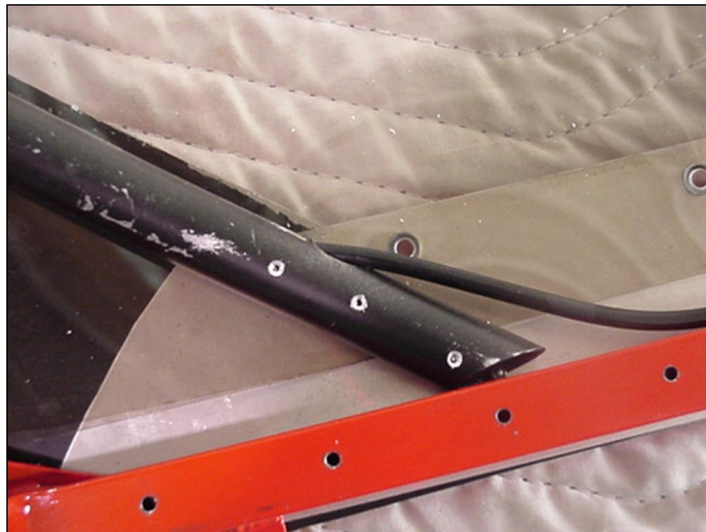
(Photo of right side showing the flexible cable housing to connect the right latch to the canopy open handle mounted on the left side).
