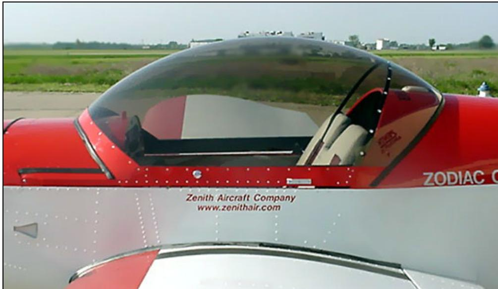
Position the canopy fore and aft: the front bottom corner is in line with the instrument panel. Check: Look at the canopy on profile to find the highest point for maximum headroom.
