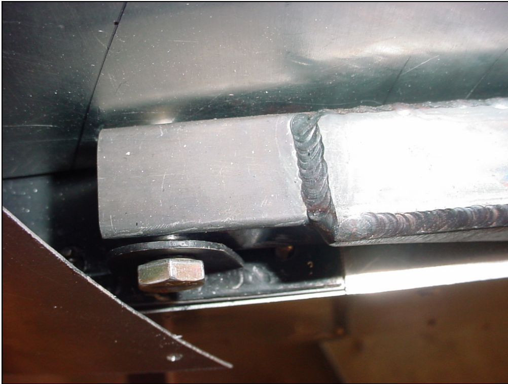
Insert the AN4 bolt for the front pivot.
