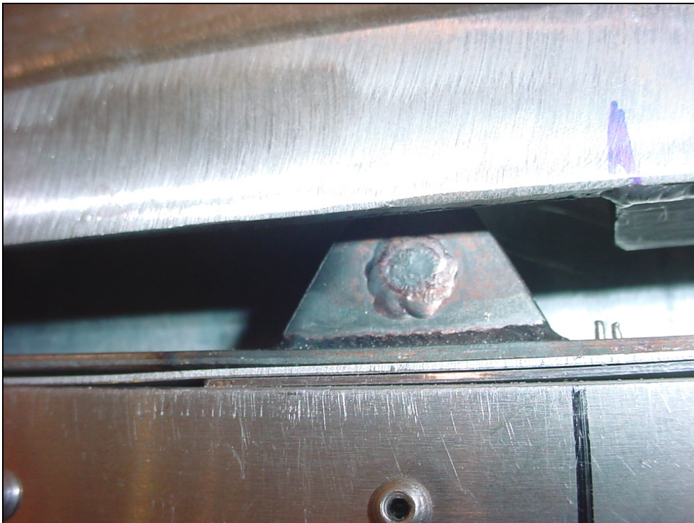
Position the bottom bracket 6C2-2 on the fuselage, the front edge is flush with the gusset 6B12-5. Ref top left diagram on drawing 6-C-1. Check that the welded plate with stud does not interfere with the square tube.
