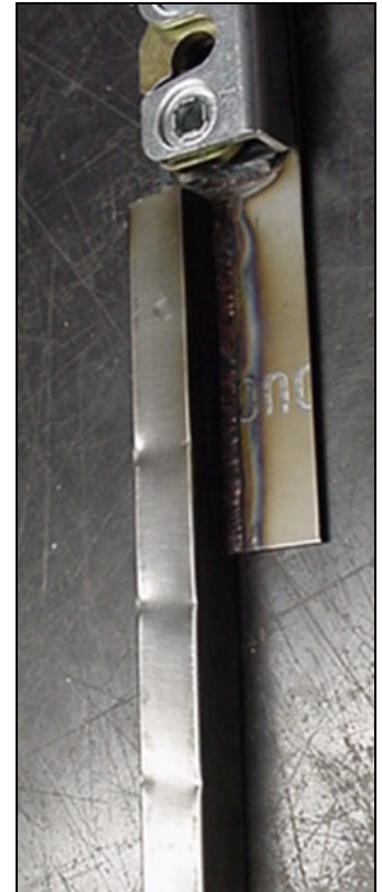
Kinks at the location of the middle bolt.
