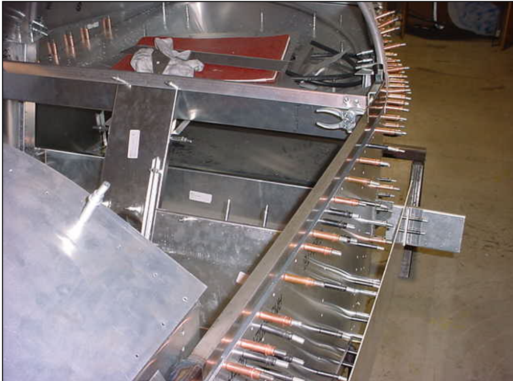
Left side. Check that the Canopy Side Frame follows the curvature of the fuselage.
