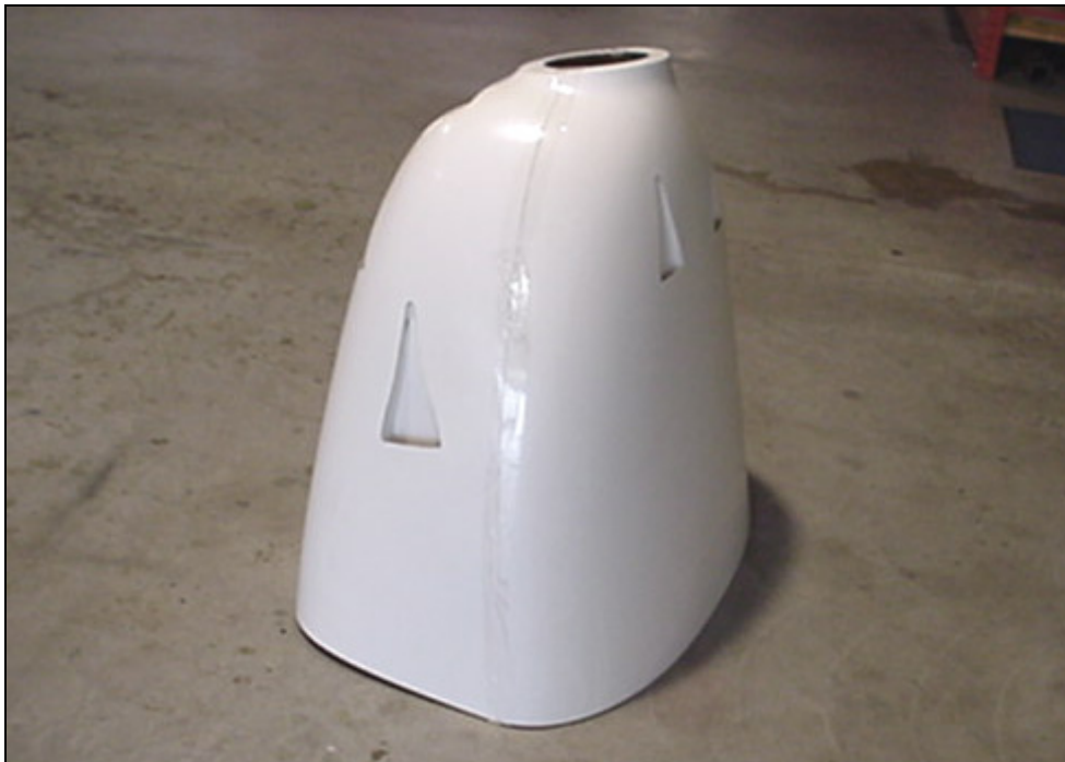
Fiberglass cowl with the NACA scoops installed.
