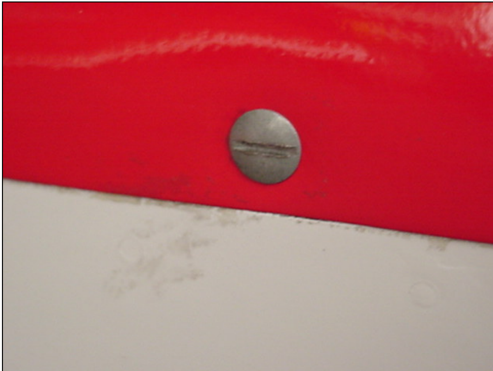
Photo of Dzus fastener to hold the top and bottom half of the cowls together.
