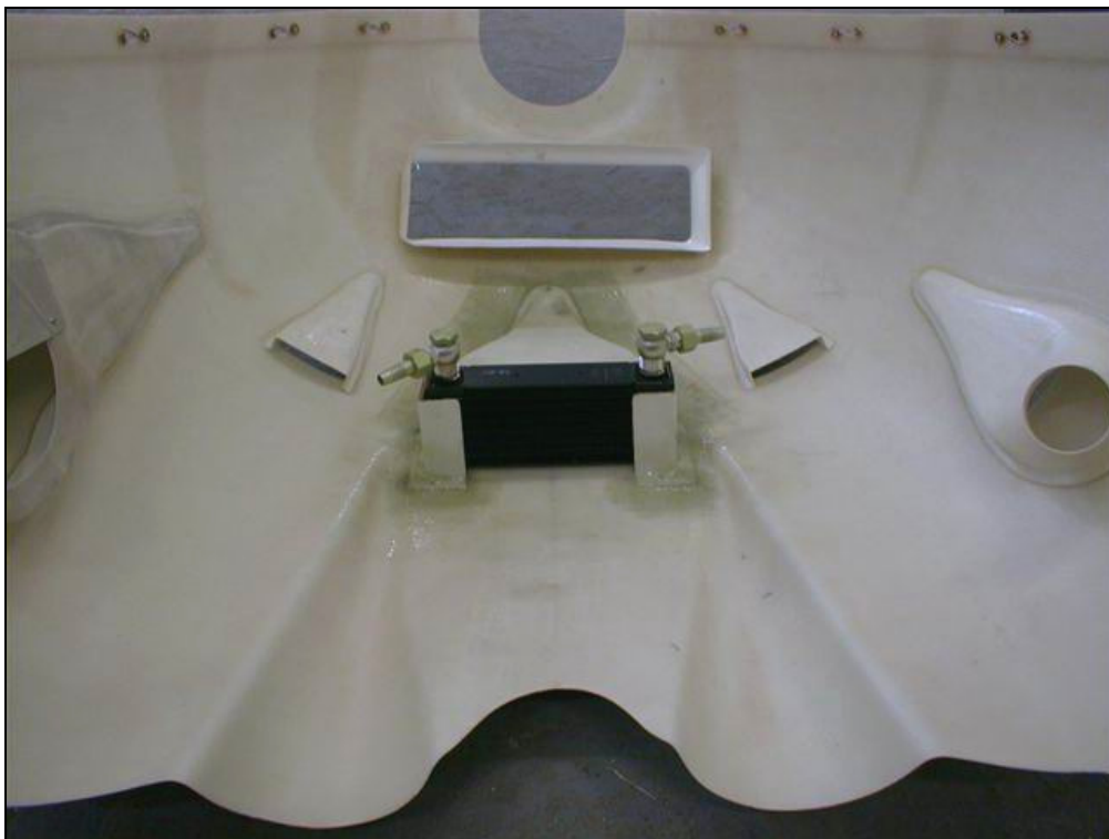
Looking inside the cowl, the oil cooler fits behind the NACA scoop.
